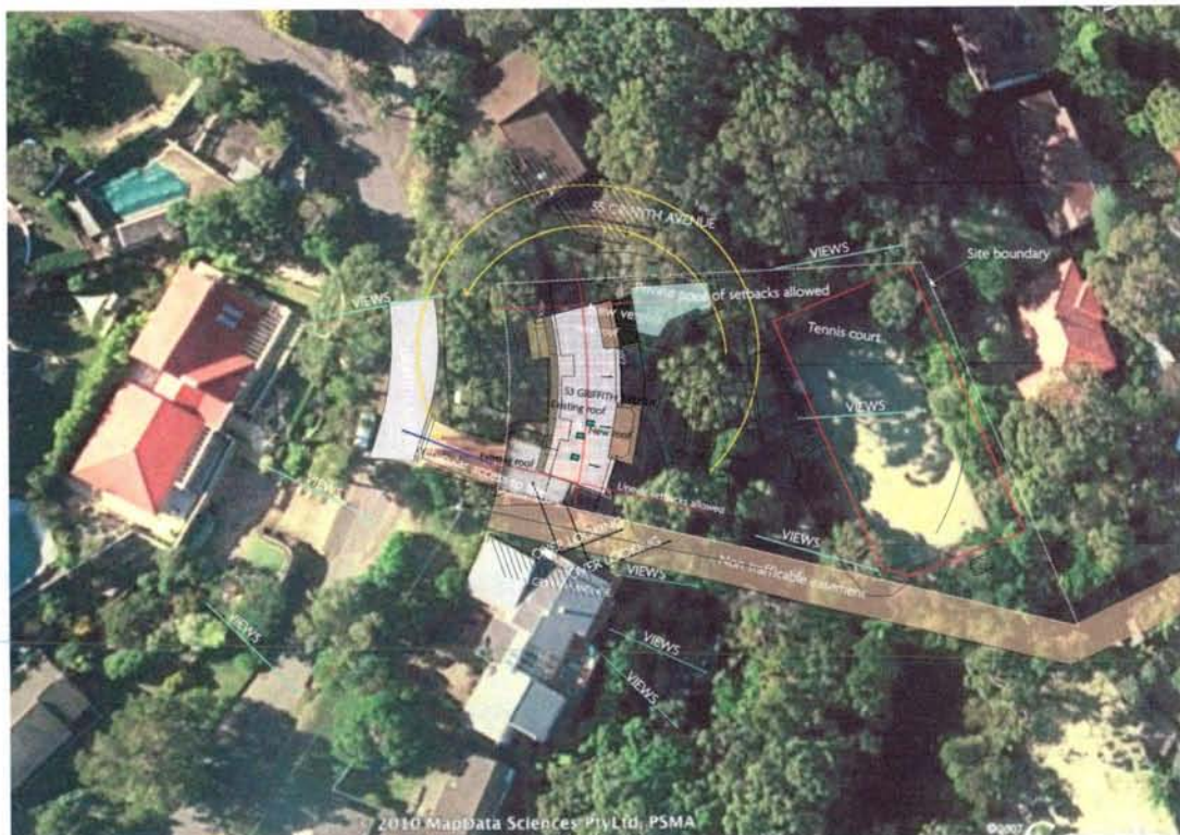
Figure 20 Aerial Site Analysis Plan above shows the solar access to the site and an overlay of the proposed design over an aerial photo of the site
