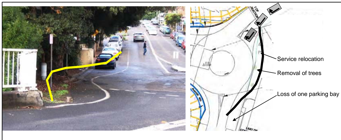
Figure 24 Southbound Bypass Lane Through Roundabout – Indicative Layout and Constraints
