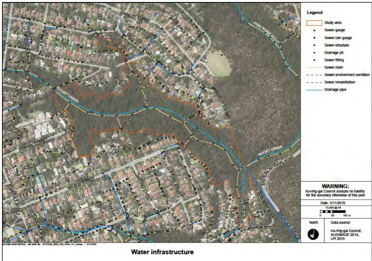
Figure 7. Location of sewer infrastructure and easements
