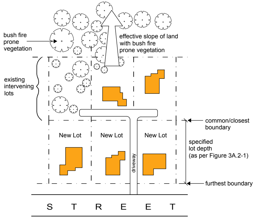
Figure 3A.2-4. Example of the recommended lot depth for new lots separated from bush fire prone vegetation by an existing intervening lot.
