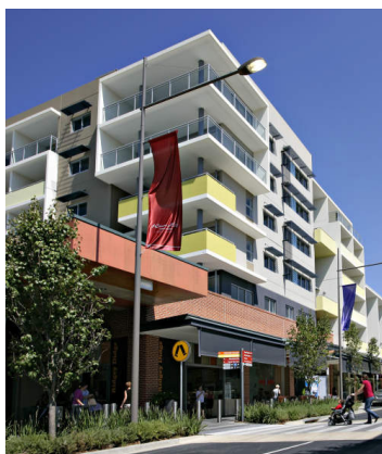
Figure 8C.14-1: Use of a mix of solid and transparent balustrades on different levels to ensure visual privacy.
