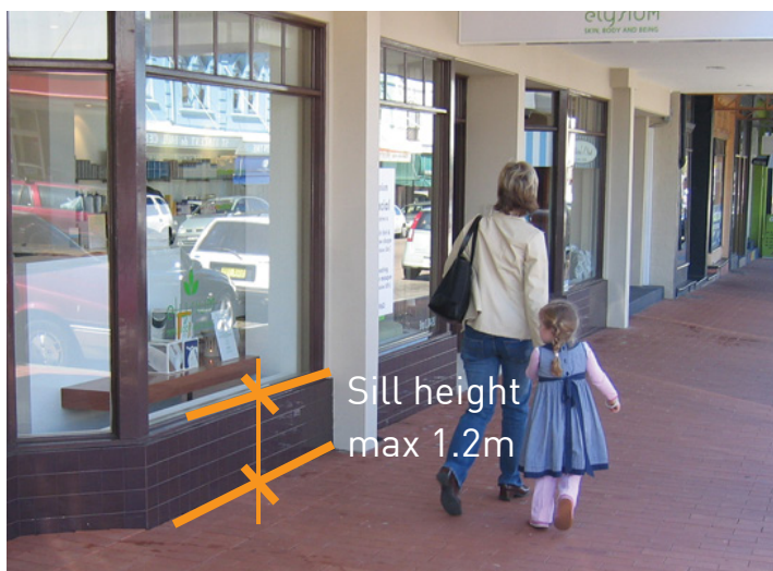
Figure 8C.10-2: Sill height controls for ground floor commercial premises to achieve an active street frontage.
