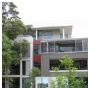
Figure 23.9-1: Balconies with sliding panels to increase visual privacy.
