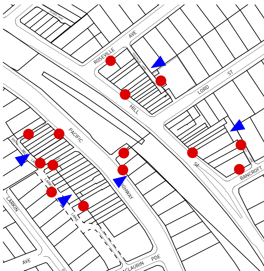
Figure 14F.6-1: Building entries, car parking and service access plan.
