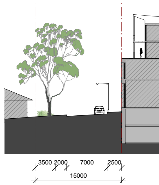
Figure 8: Balfour Lane re-alignment street section
