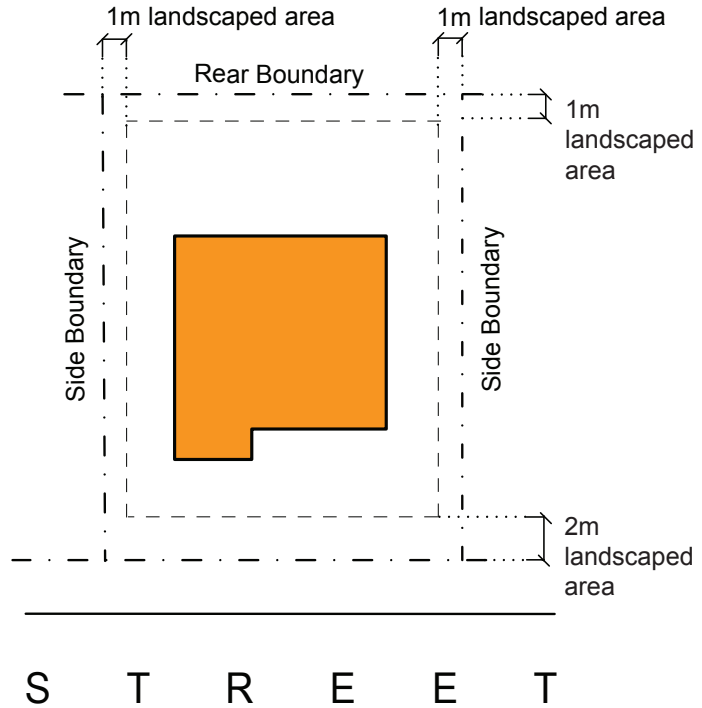
Figure 10A.3-1: Single frontage sites: minimum landscaped area for low density residential areas
