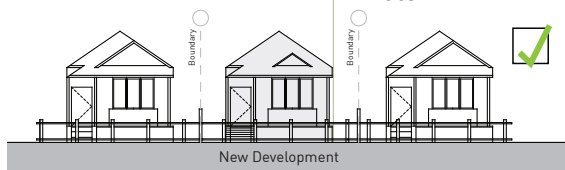
Figure 19C.8-1: Good design: New development uses similar fencing detailing to existing.
