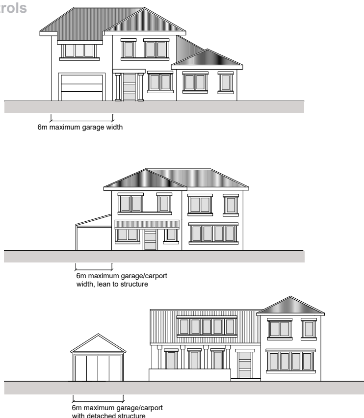
Figure 4B.3-1- Maximum widths of garages and carports
