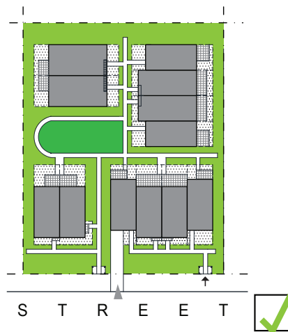
Figure 6A.2-3: Site layout with >25m frontage.
