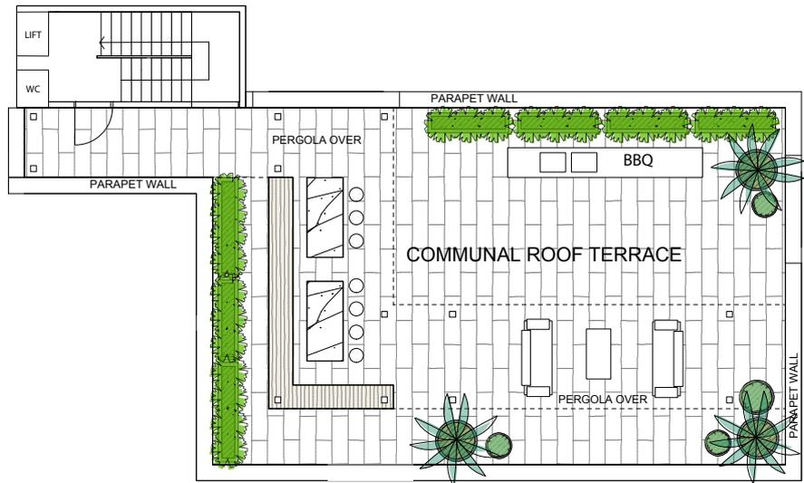
Figure 23.5-5: Roof terrace design
