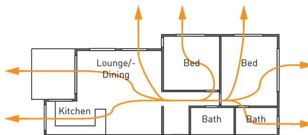
Figure 6C.4-1: Building layout that facilitates cross ventilation.
