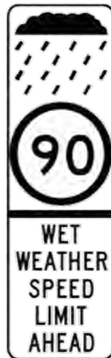
Figure 22 – 'Wet weather speed limit ahead' sign (R6-249)
