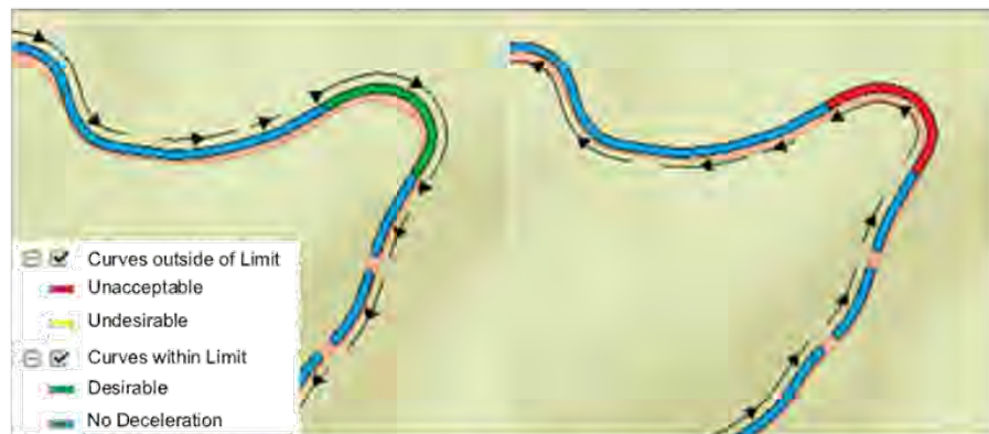
Figure 3 – Example of curve analysis on Alpine Way, NSW in southern direction (left) and northern direction (right) (Source: Transport for NSW)
