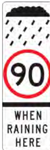
Figure 23 – 'Speed restriction – when raining here' sign (R4-238N)
