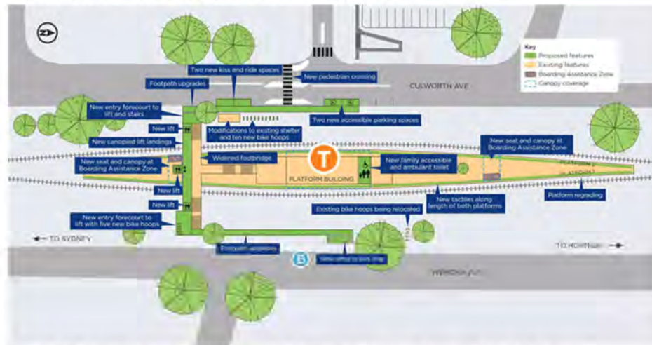
Figure ES- 1 Key features of the Proposal (indicative only - subject to detailed design)
