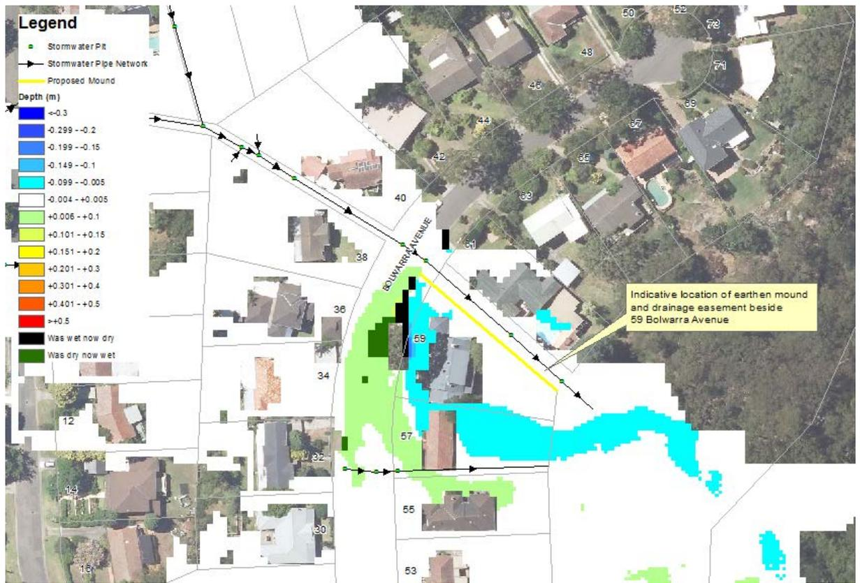
Figure 8-10 Option FM5 20% AEP Change in Water Level
