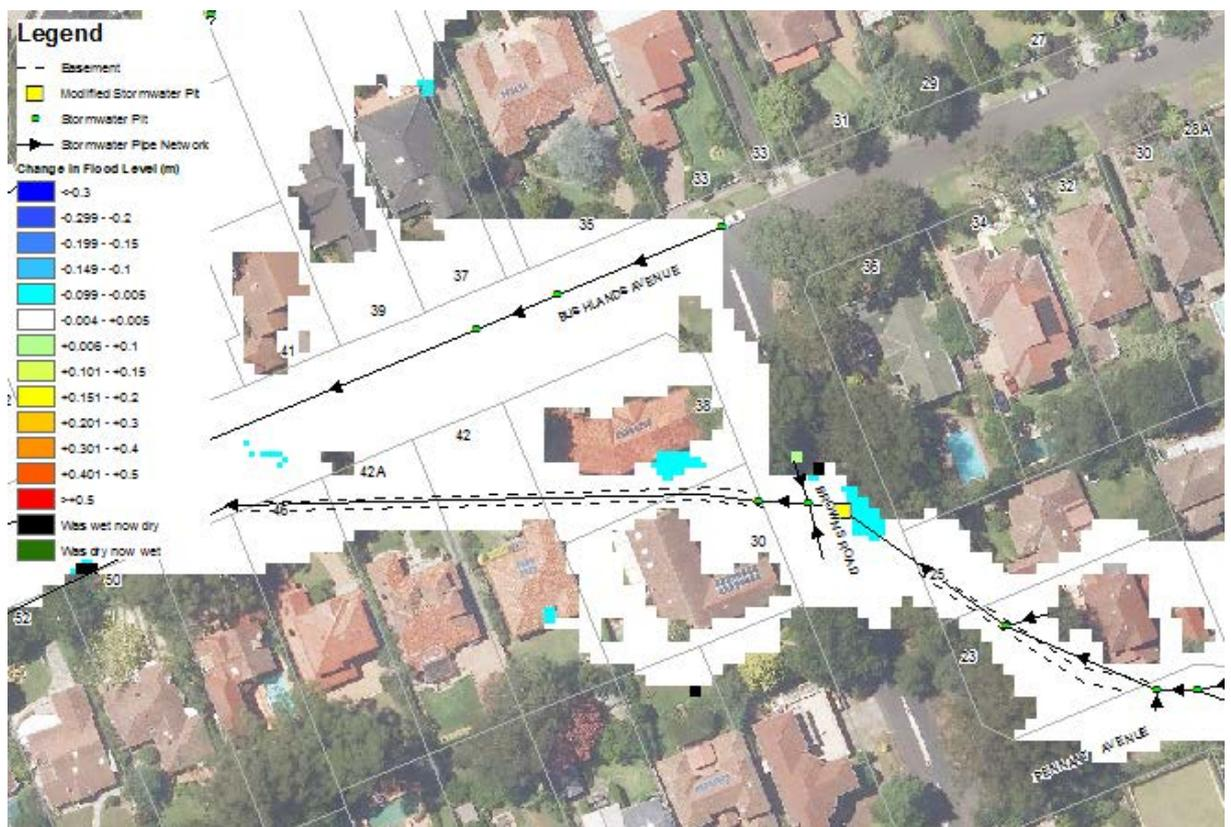
Figure 8-21 Option FM9 1% AEP Change in Water Level
