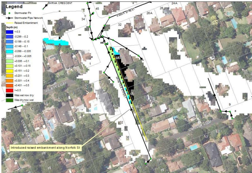
Figure 8-7 Option FM4 20% AEP Change in Water Level
