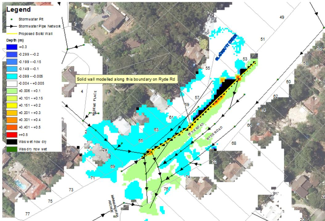
Figure 8-19 Option FM8 1% AEP Change in Water Level
