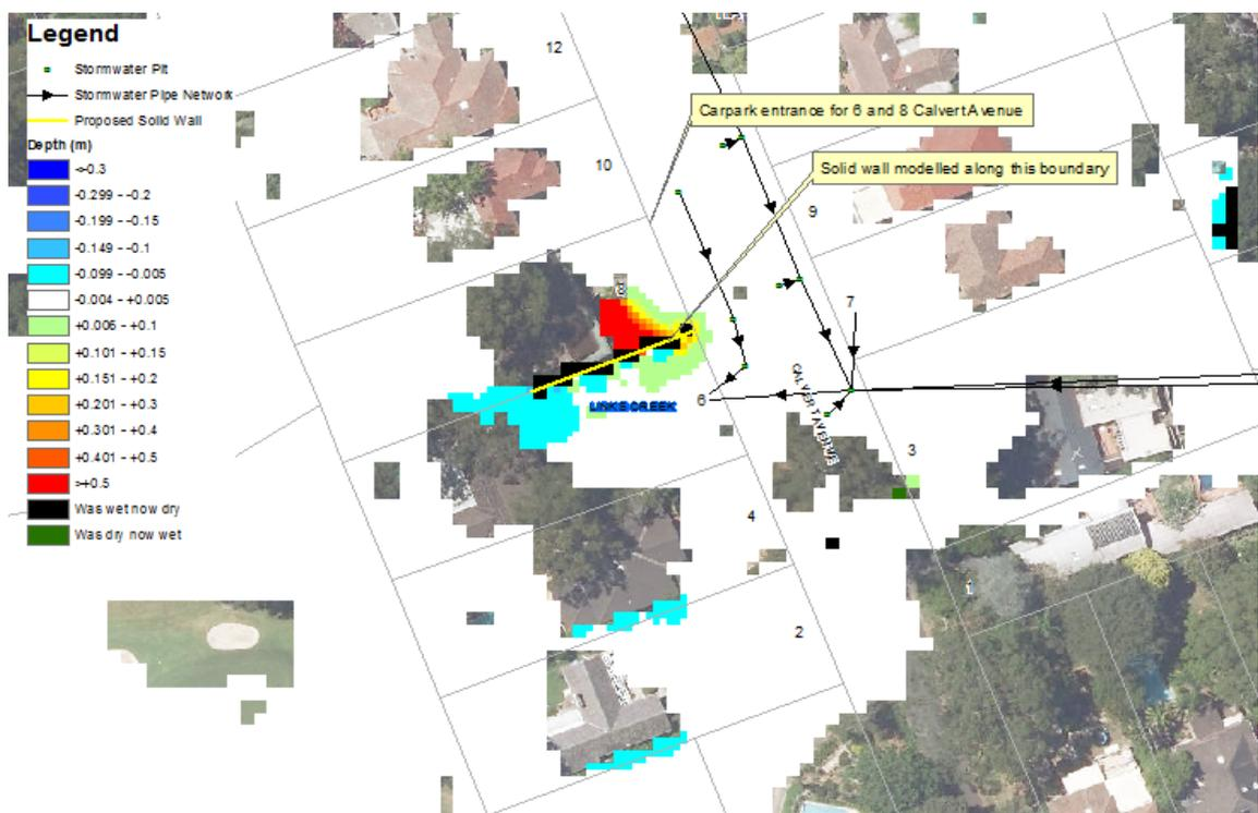
Figure 8-16 Option FM7 1% AEP Change in Water Level
