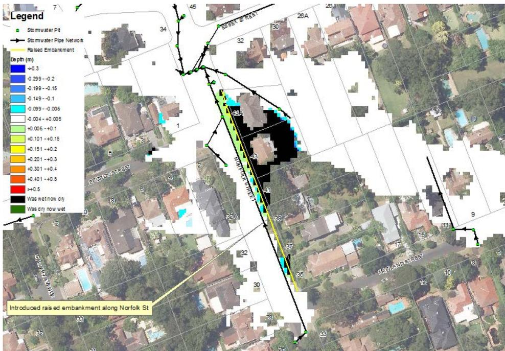
Figure 8-8 Option FM4 1% AEP Change in Water Level
