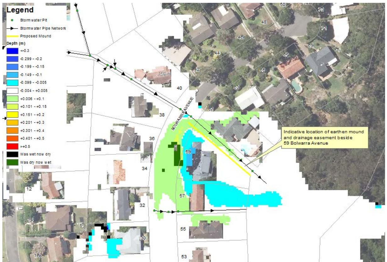
Figure 8-11 Option FM5 1% AEP Change in Water Level
