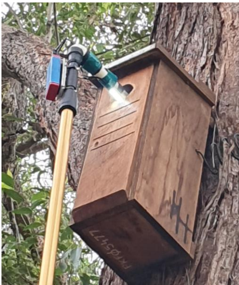
Example: MK3 camera inspecting a nest box
