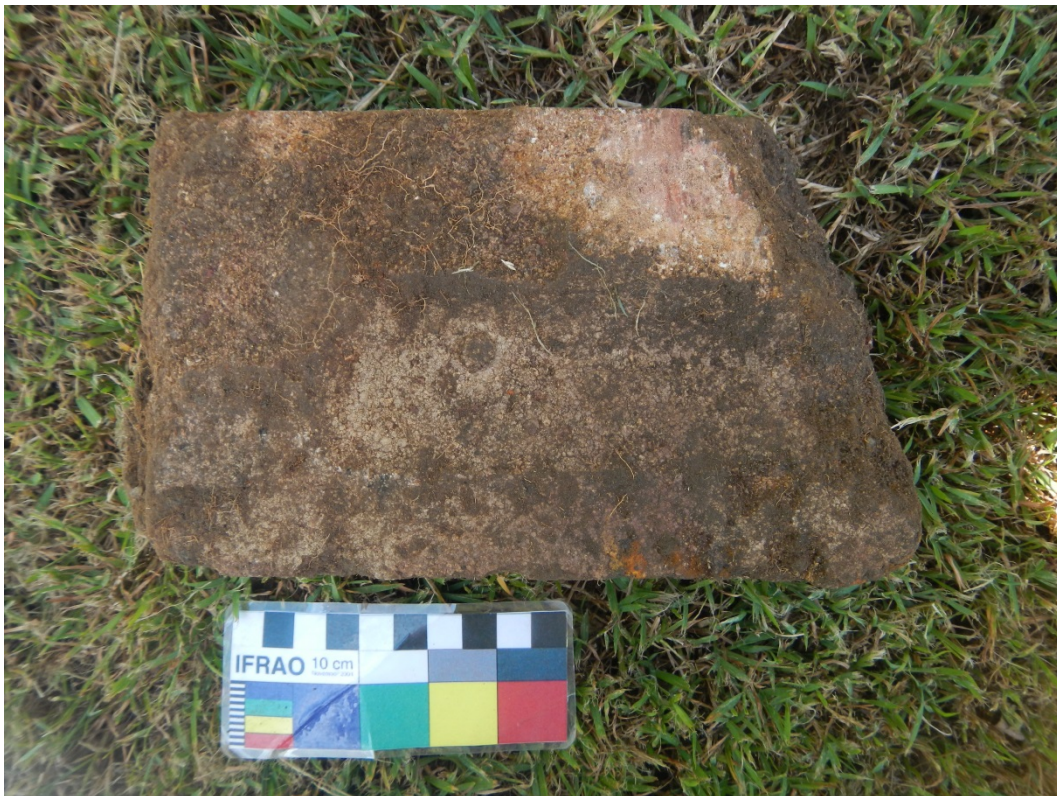
Figure 6. Machine pressed brick with frog and screw impression from TP3.
