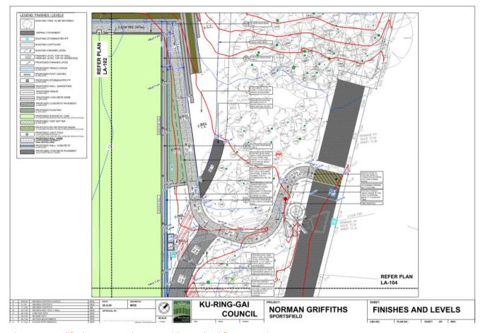
Figure 9 - Modified eastern paths to provide overland flow capacity
