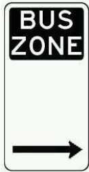
Figure 3.6-1: Typical bus zone sign.
