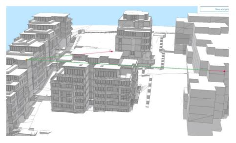
Slice – display a vertical or horizontal cross section of a building development.
