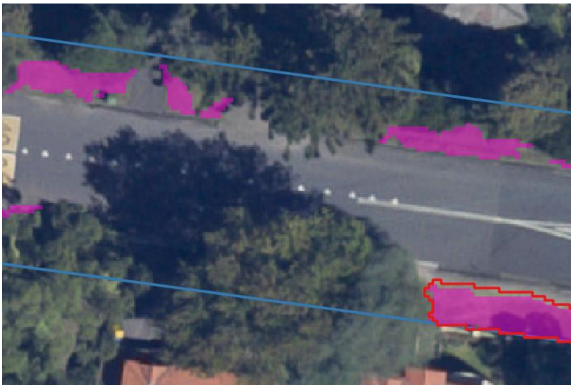
Figure 7: Narrow slivers of potential planting space (purple) excluded from final available planting space (APS) dataset (red) due to being too narrow to support additional trees, with road boundaries (blue) as an overlay.
