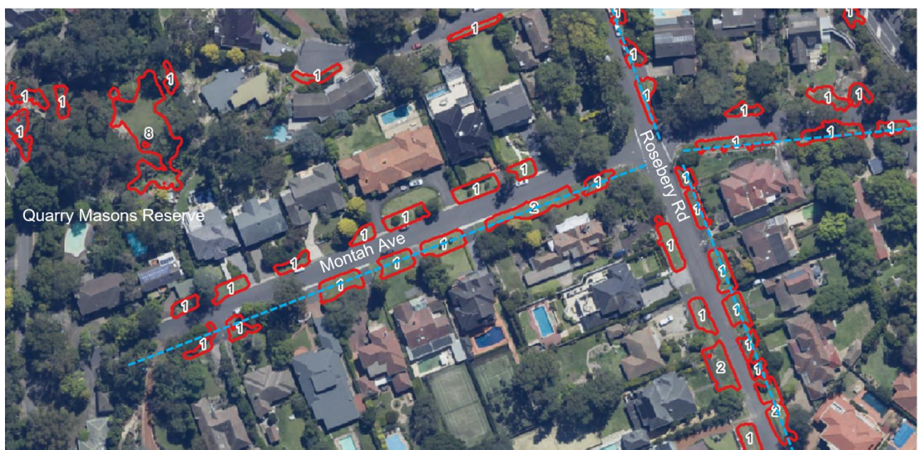
Figure 15: Example of APS dataset, showing identified APS in red, and the number of trees that could fit in the available space (label). Overhead power distribution lines observed in the aerial imagery is illustrated as a dotted blue line.
