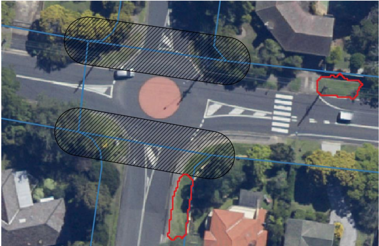
Figure 6: Exclusion zones (black hatched) around road boundary (blue) intersections used to exclude available planting spaces (APS; red) from within 10m of projected line of the intersecting kerb line. Note the offset between road intersection line in exclusion zone and the actual road surface intersection.
