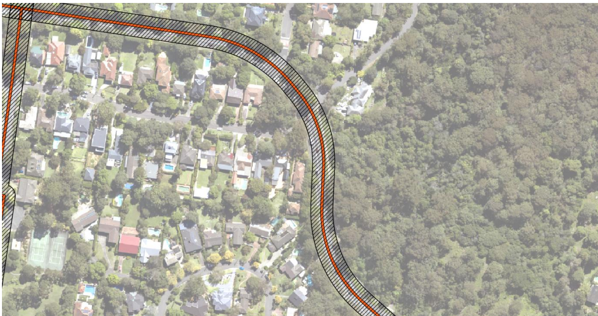
Figure 11: Inaccuracies in cycle route vector dataset (orange line), with route on the far eastern side of the road in the north of the scene and along the centre of the road toward the south of the scene. The buffered 10m boundary used for shade modelling analysis is shown in a black hatched pattern.
