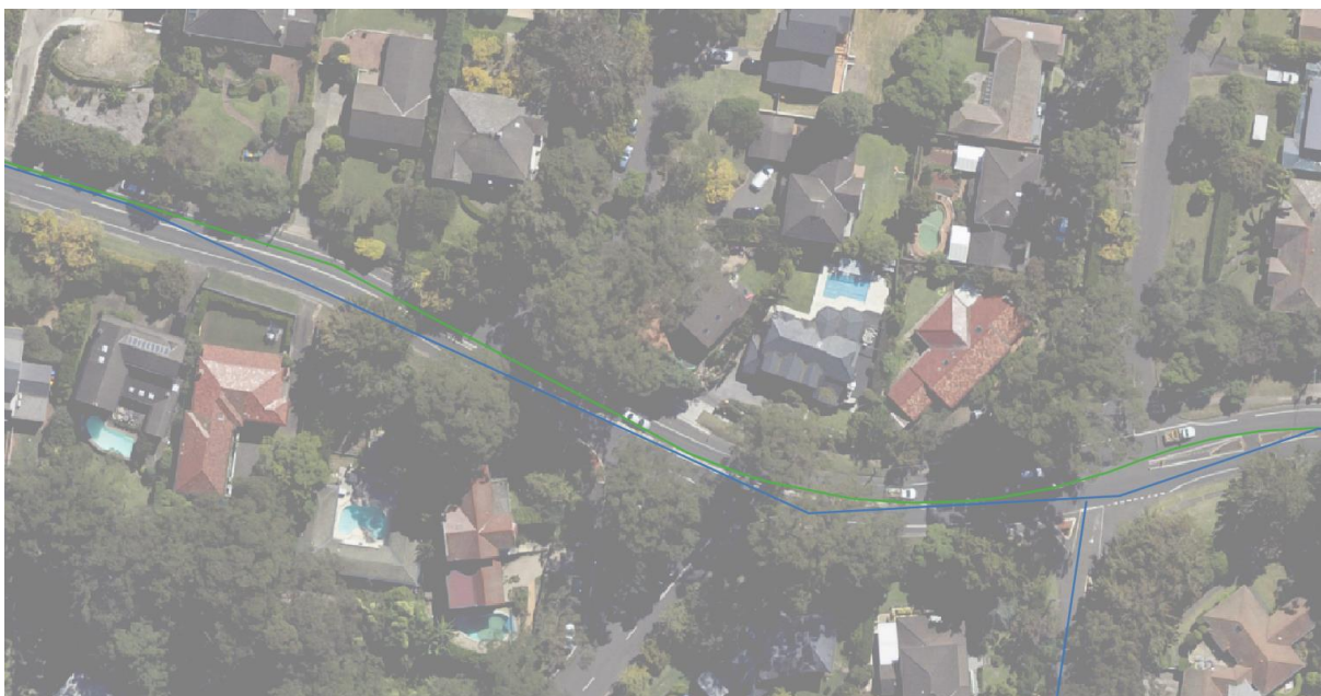
Figure 9: Duplicate cycle route appearing in both the existing (green) and proposed (blue) cycle route vector datasets supplied by the Council prior to consolidation to a single cycle route to simplify analysis and management.
